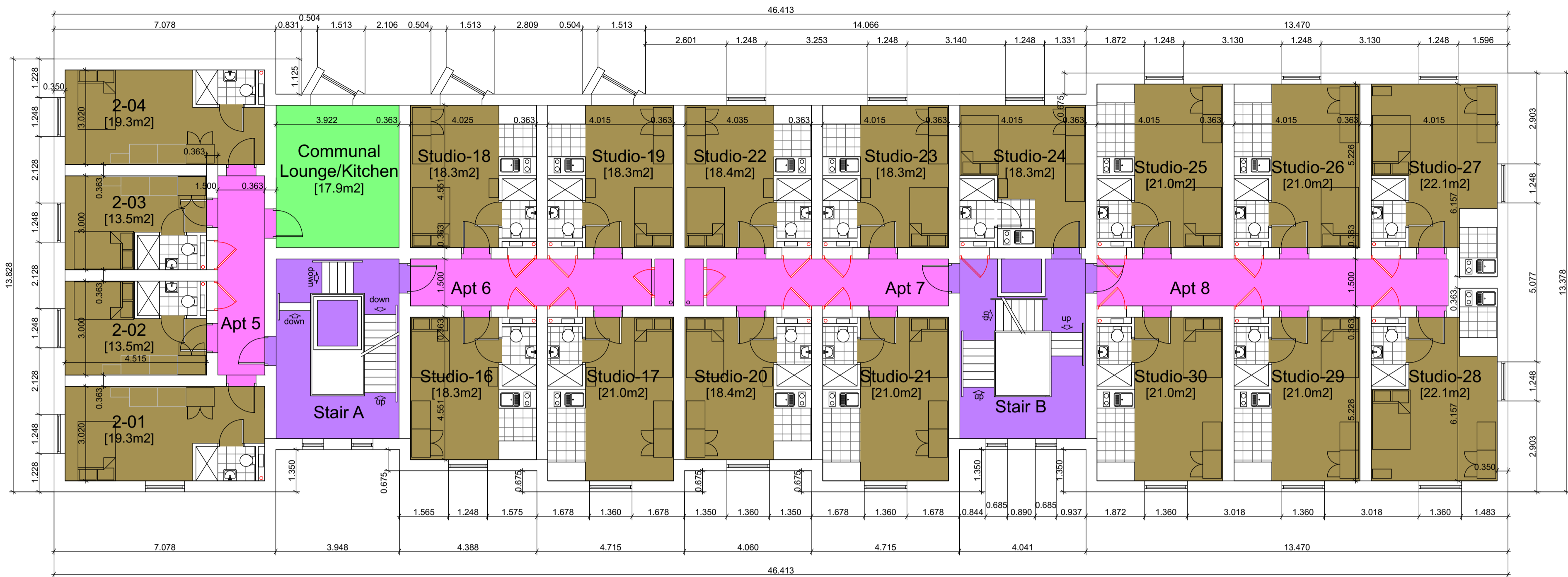
PROPOSED FIRST FLOOR PLAN Areas shown in [brackets] are Approx Gross Internal Floor Areas
