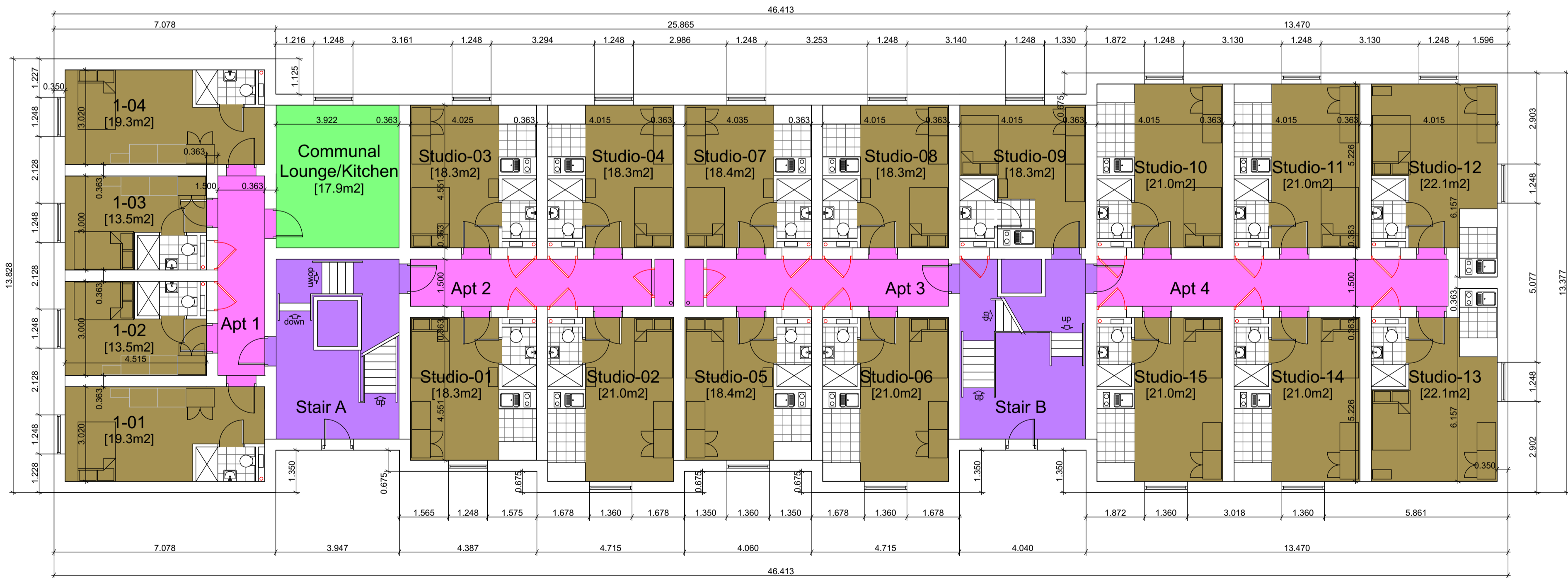
PROPOSED GROUND FLOOR PLAN Areas shown in [brackets] are Approx Gross Internal Floor Areas
